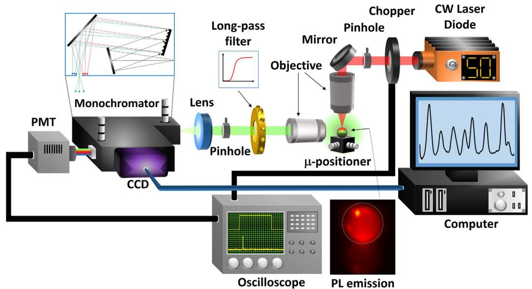
**Figure 1. Schematic diagram of the experimental set-up.** Dimensions are not to scale. The bottom-right panel illustrates a spatial profile of the emitted PL below lasing threshold, which has been taken by placing the focus of the collection objective at the sphere center and widely opening the pinhole. The sphere contour is highlighted for clarity. The bright spot is probably associated to a scattering region within the sphere. The figure has been drawn by J. M. Ramirez.
