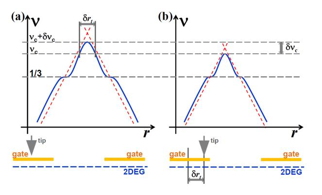
A displacement  $\delta r_t$  of the SGM tip toward the QPC center reduces the QPC width of the same amount. The corresponding reduction of the filling factor at the QPC center (which is measured as a reduction of  $G_T = vG_0$ ) is approximately given by  $\delta r_t/2$  times the filling factor slope.
