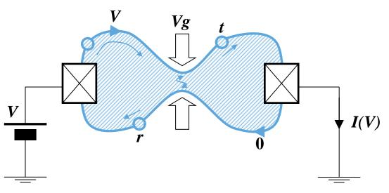
With a QPC we can intentionally induce backscattering, which provides us information about the edge properties
