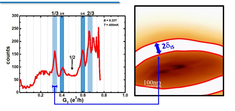
The incompressible stripe width  $\delta_{\rm IS}$  is obtained starting from the FWHM of the corresponding peak in the histogram (left panel). This range of  $G_{\rm T}$  values defines a circular stripe in the SGM map (right panel).  $\delta_{\rm IS}$  is given by the average width of such a stripe.
