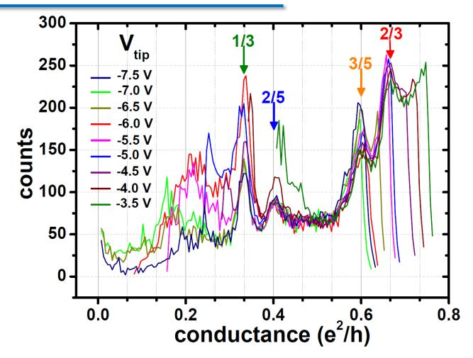
Histograms of the occurrence of each  $G_T$  value for all the 9 different SGM scans performed at different  $V_{tip}$  values. Fractional peaks are visible in each individual histogram.
