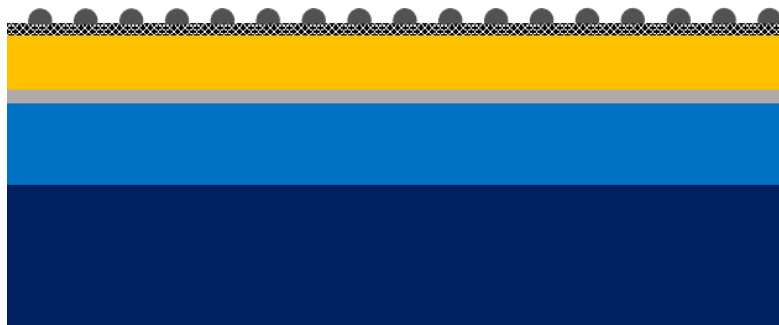
Figure 2.3: Scheme of the sensor (dimensions not in scale). From the top: Ti evaporated (dark gray islands), graphene monolayer (black and white), Au layer (yellow), Ti layer for proper sticking (gray), \text{SiO}_2 insulator layer (light blue), Si substrate (dark blue)
