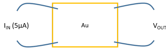
Figure 3.11: Scheme of the 4-wire setup which allows to directly measure the actual sensor resistance. We supply the sensing current using the TC contacts and we read the voltage drop using the add contacts.
