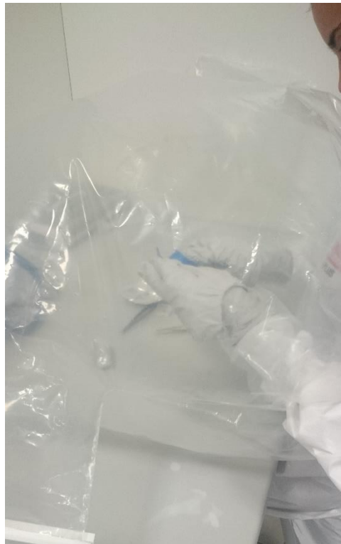
Figure 9:Glove bag's picture. The bag is filled with nitrogen and we exfoliate black phosphorus inside.
