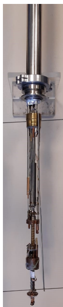
Figure 44: Bottom part of the insert system, still uncovered. The floating metal rod on the right is the capillary.
